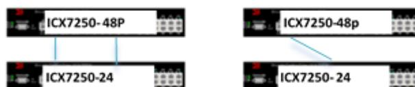
**Four unit stack linear and ring topology**
