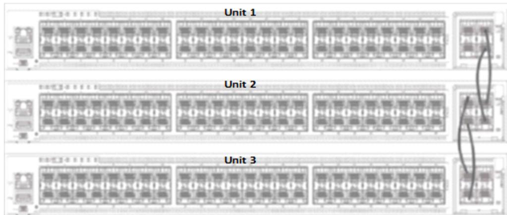
**TABLE 4** Stacking connections in Brocade ICX 7450 three unit stack
